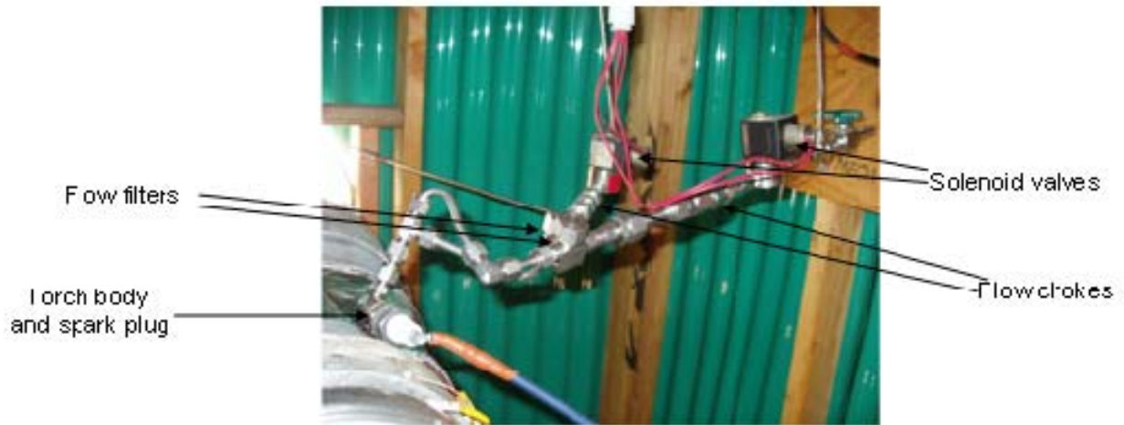
Figure 11. Ignition System Illustration
