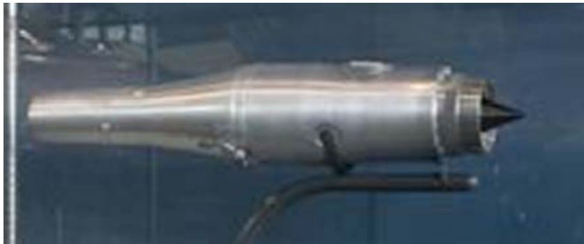
Figure 4. Illustration of Williams International F-121 Fanjet
