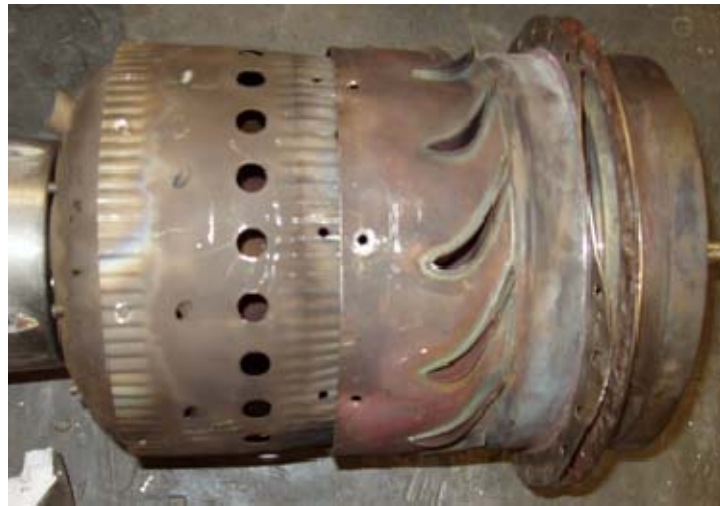
Figure 5. Illustration of the Turboméca Piméné type combustor inside the F-121 fanjet engine.
