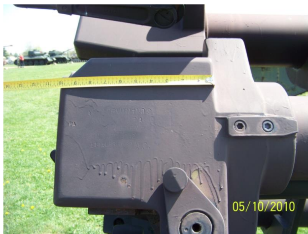
Figure 2 Measuring the M1 Test Gun breech (Aberdeen Ordnance Museum)
