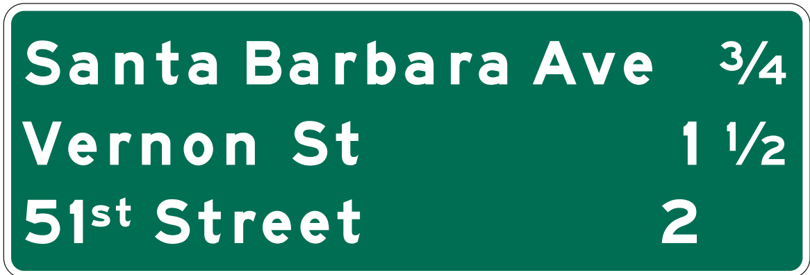
Figure 2E-24. Interchange Sequence Sign
