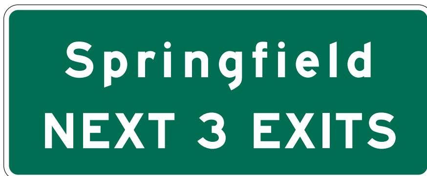
Figure 2E-26. NEXT EXITS Sign
