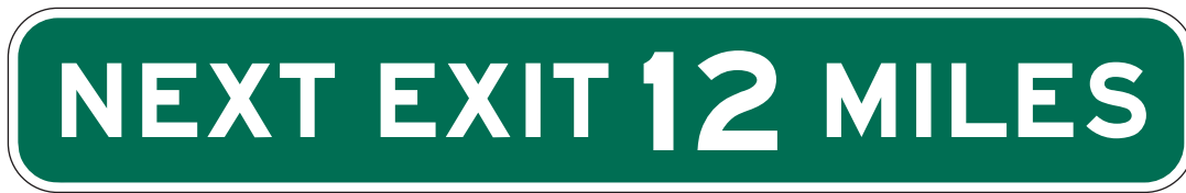
Figure 2E-16. Next Exit Supplemental Advance Guide Signs
