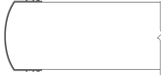
4 x 4 COPPER CAP SIDE ELEVATION
