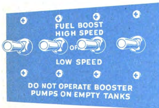
FUEL BOOSTER PUMP SWITCHES
