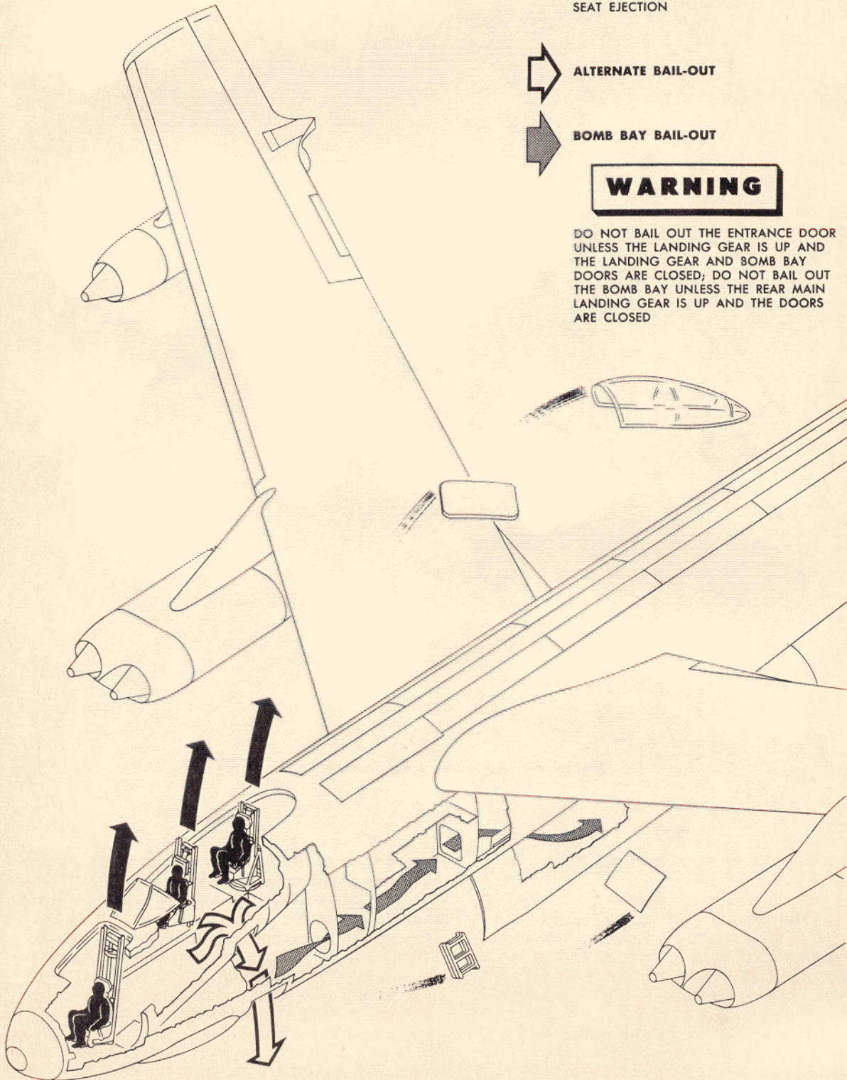
Figure 3-2 (Sheet 1 of 2 Sheets). Emergency Exits and Entrances
