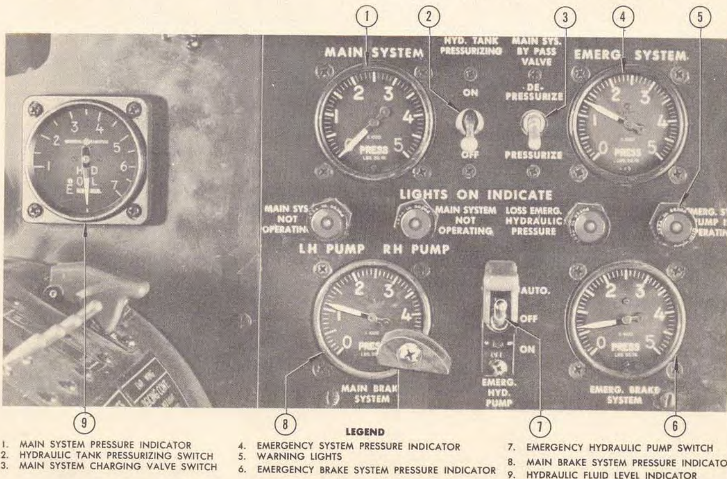
Figure 1-20. Hydraulic Control Panel
