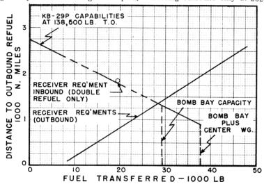
nautical miles or refueling outbound at 675 nautical miles and inbound at 1845 nautical miles; however, reading from the requirements section, the double refuel requires two tankers, one outbound at 675 nautical miles transferring approximately 17,500 pounds fuel and inbound at 1845 nautical miles transferring 19,350 pounds fuel.
