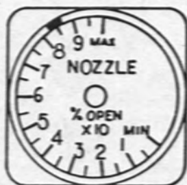
PRIMARY EXHAUST NOZZLE POSITION INDICATOR (6)
