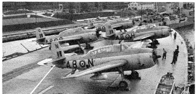
Avengers of VS 881 being used to pull HMCS Magnificent off the jetty.
