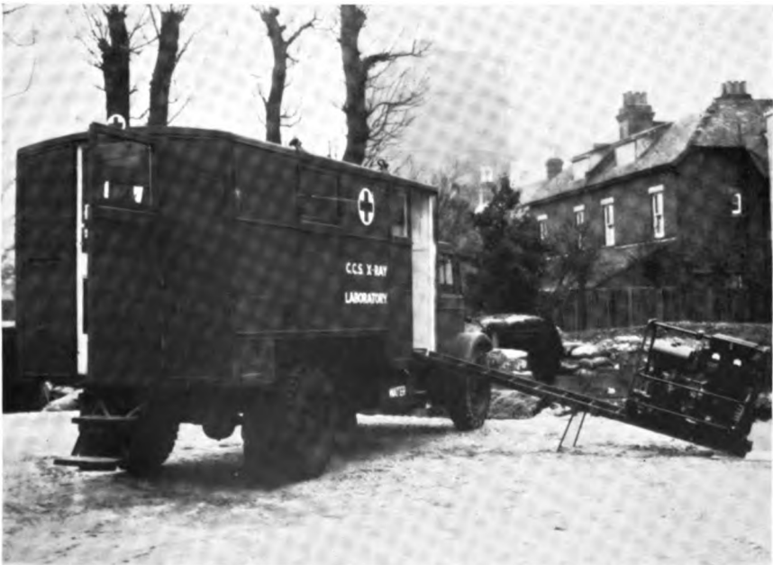
PLATE XXV: C.C.S. X-ray Laboratory and Generator, 1939. From 1940/41 5 k.v.a. Petro-Electric Alternators 230 v., a.c., were supplied.
