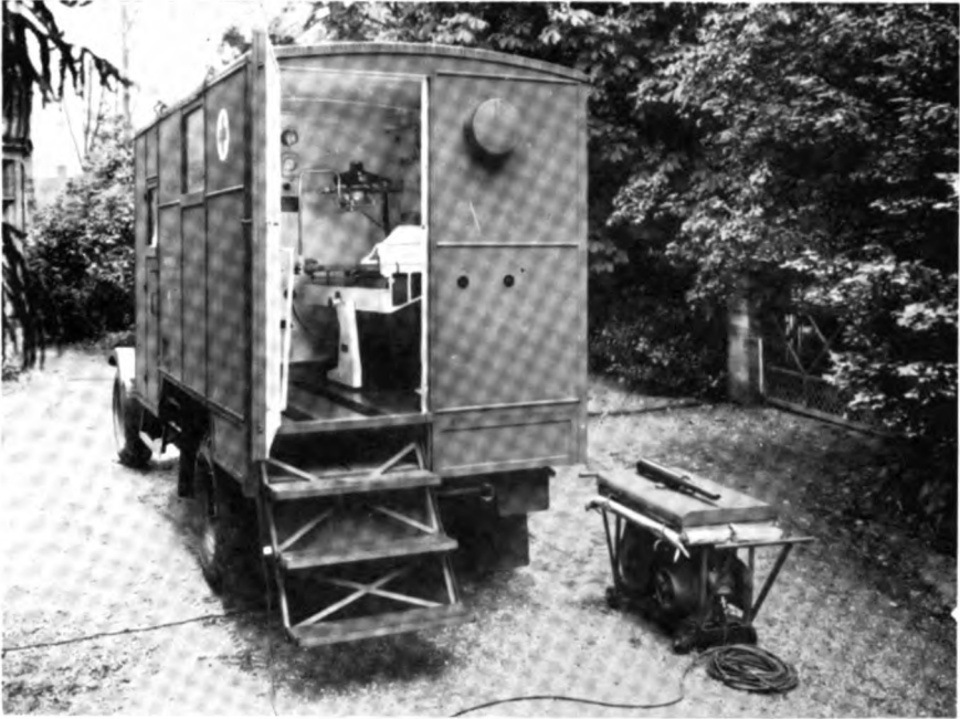
PLATE XXXVI: Michaelis Field Unit with generator showing tilting tube, etc., inside
