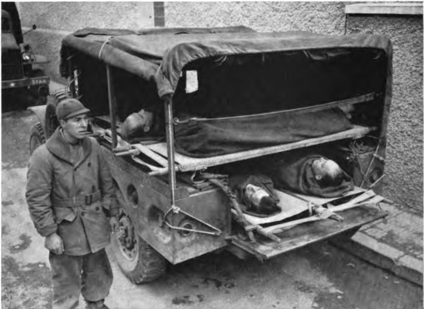
PLATE XXI. A 3-ton Weapons Carrier used for the evacuation of casualties. Three stretchers on top tier, two below.
