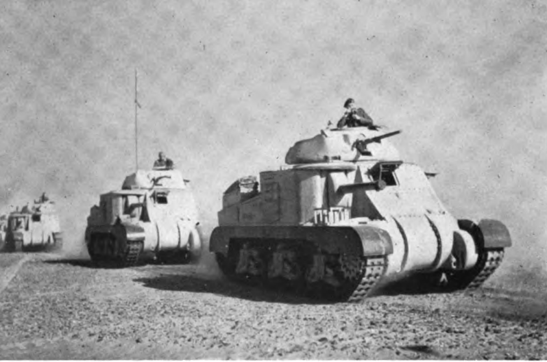
12. The American Grant, mounting a 75-mm gun in a sponson and a 37-mm high velocity gun in the turret.
