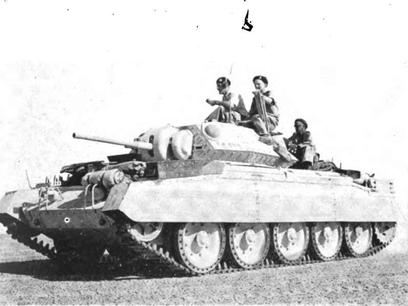
13. British built cruiser Crusader; like Matilda and Valentine, it mounted a 2-pdr gun in a revolving turret.
