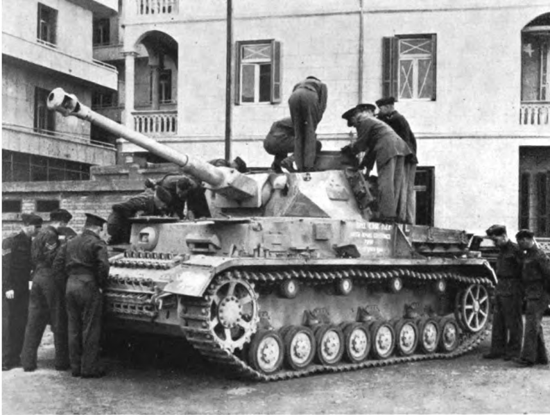
18. Pzkw IV Special, with its powerful long 7.5-cm gun. One of the few to be taken intact.
