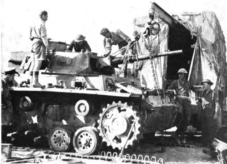
16. Pzkw III Model H with short 5-cm gun and extra plate on the front superstructure; the first of such tanks to be captured being dismantled for examination, May 1941.
