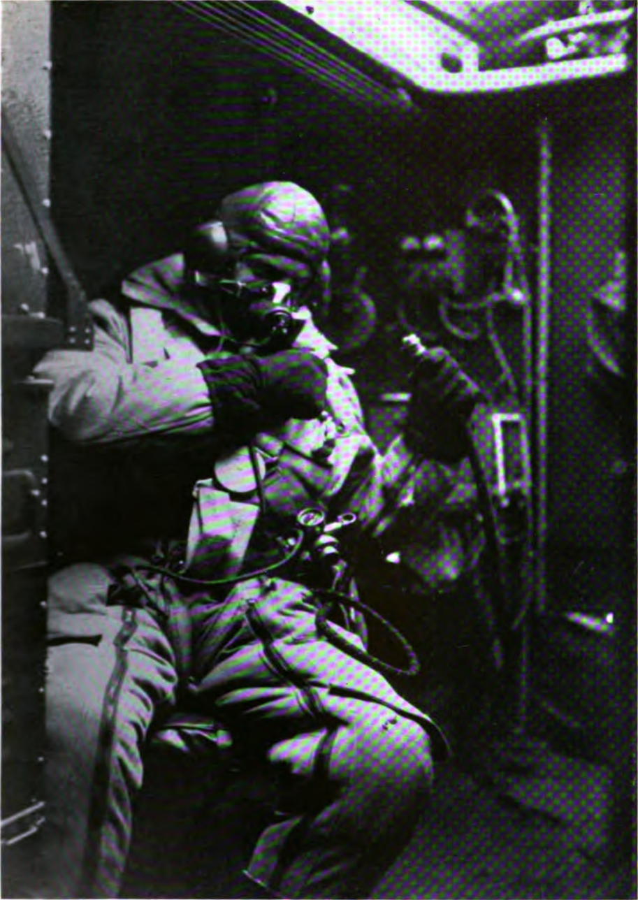
PLATE X (a): Uncoupling the Main Oxygen Hose prior to attaching the Portable Apparatus
