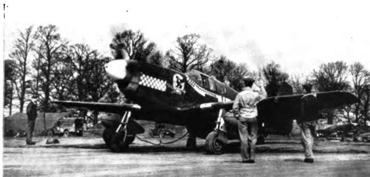
4. A P-51-B Mustang of the United States 8th Air Force being prepared for operations against Brunswick on 8th April 1944. The drop tanks can be seen under the wings.
