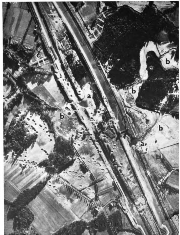
11. The Ladbergen section of the Dortmund-Ems Canal after the attack on the night of 23rd September 1944. This photograph was taken on 2nd October. Two direct hits by 12,000-lb bombs are marked a . Four points where the water has flooded over the broken embankments are marked b . The camouflaged River Glane is marked c .
