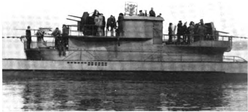
U.441 (A Type VII C, 770-ton Atlantic boat) fitted with special A.A. armament, armoured conning tower, and radar search receiver for work in the Bay of Biscay.
