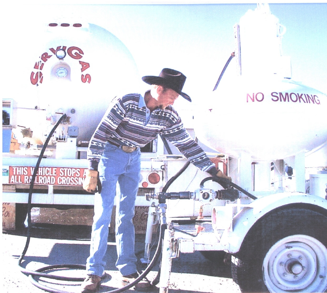
Fig. 1. A New Mexico Weights and Measures Inspector tests a Liquefied Petroleum Gas Meter to determine its compliance with NIST Handbook 44 requirements.
