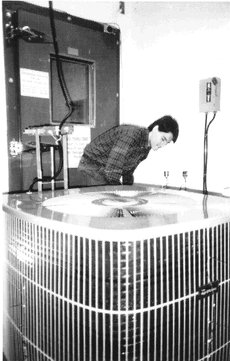
Fig. 3. Brian Dougherty prepares super-efficient heat pump for tests.
