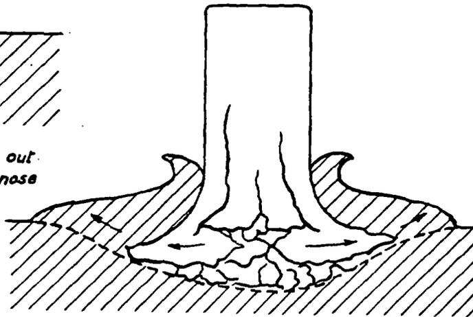
(d) Further mushrooming of shot scoops out a shallow impression as indicated by dotted line. Fragments of nose left embedded. Base of shot complete, but with longitudinal splits.
