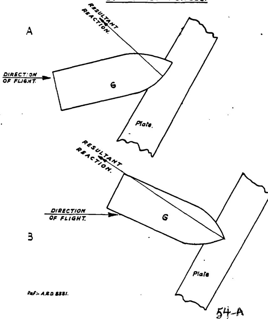
the amplitude of the yaw on impact. The angular velocities possessed by the projectile immediately before impact due to its yawing motion in air are so small compared with those arising on impact that they can be neglected.
