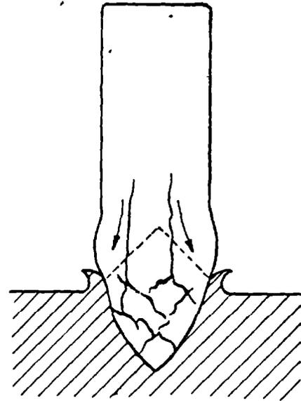
(b) Shot sets up by shear over conical surfaces, then splits longitudinally. Cracks extend into the head.
