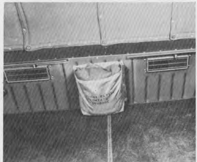
Figure 60—Heat Registers in Radio Compartment (B-24J)
