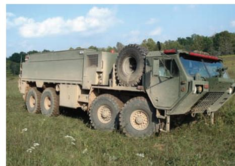
With a 2,500-gallon (9,463-l) water tank and maximum speed of 62mph (100 kph), the HEWATT can be counted upon to distribute water in the harshest environments.
