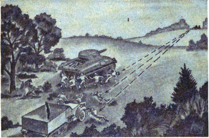
FIGURE 8.—Do not attempt to repair vehicle in the open when it can be towed to cover.
