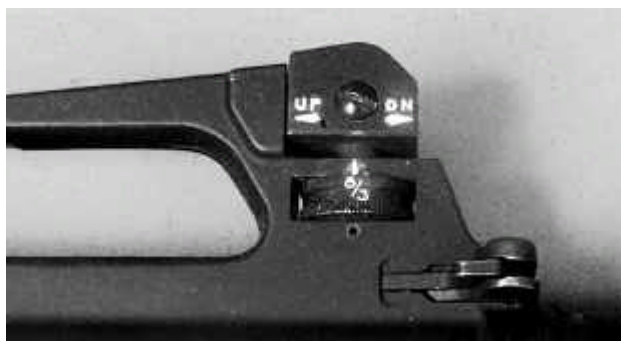
Figure 9-7. Rear Sight Elevation Knob Set for 800 Yards/Meters.
