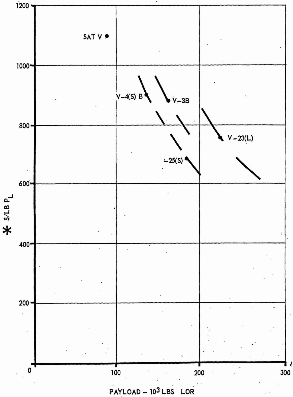
Figure 21. Three-Stage Payload Cost Efficiency.
