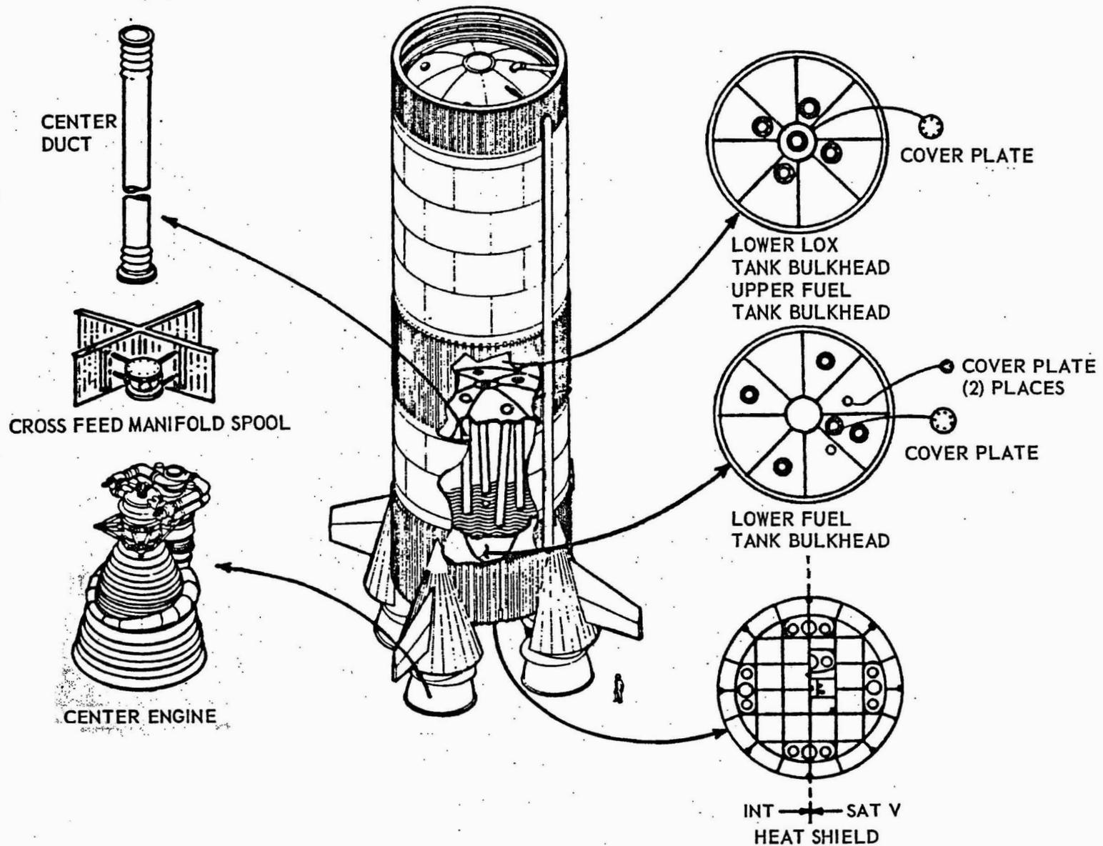
Figure 2. Four Engine INT-S-IC Stage.
