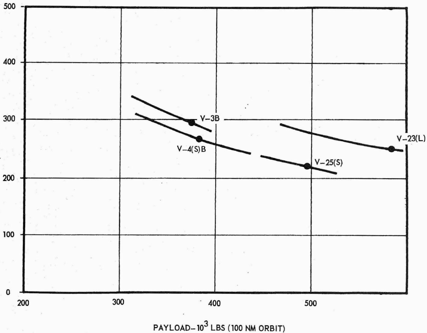
Figure 20. Two-Stage Payload Cost Efficiency.
