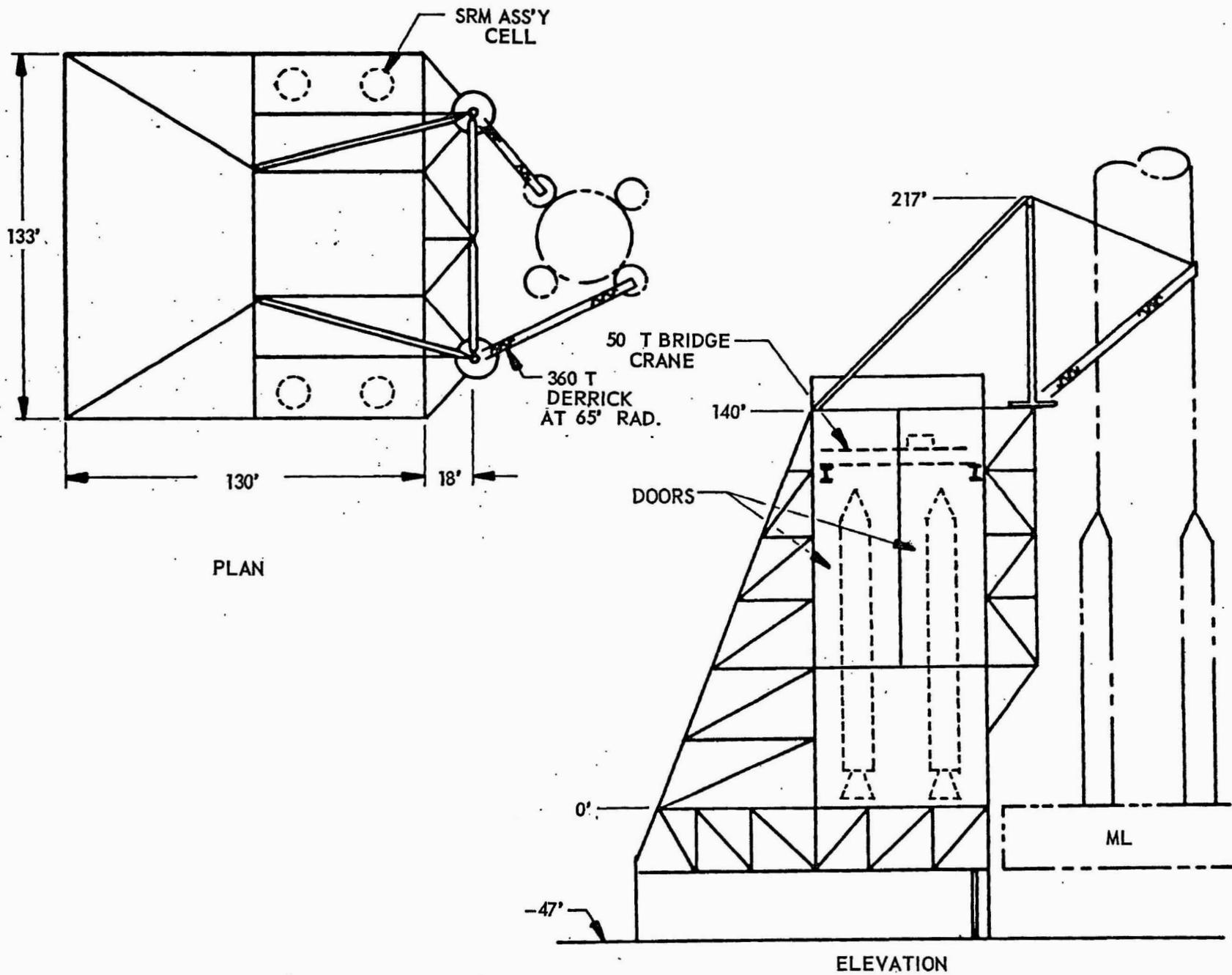
Figure 13. Mobile Assembly and Handling Structure.
