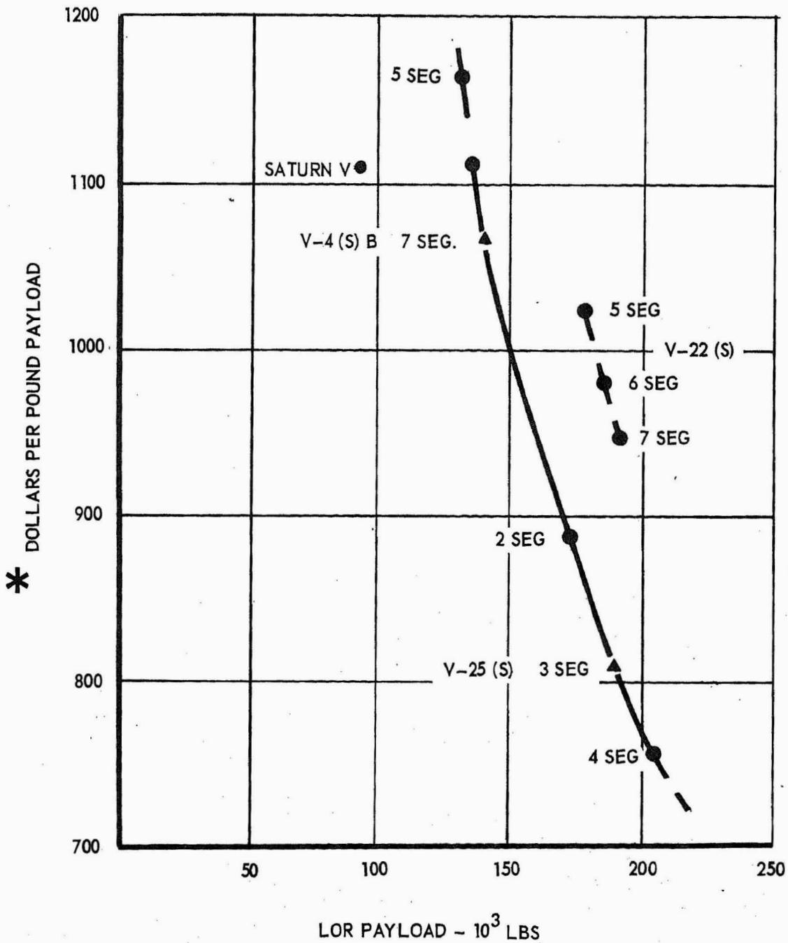
Figure 9. SRM Boost-Assist Cost Efficiency Comparison.
