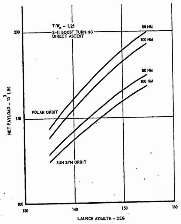
POLAR AND SUN SYNCHRONOUS ORBIT PAYLOAD CAPABILITY
