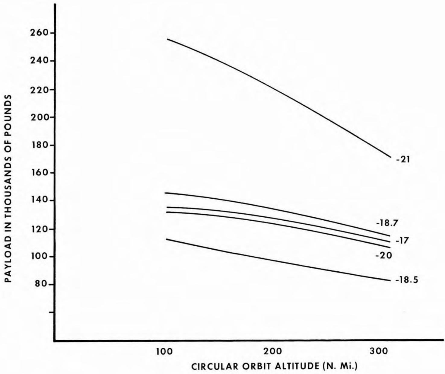
FIGURE 14 INTERMEDIATE VEHICLES CIRCULAR ORBIT PERFORMANCE
