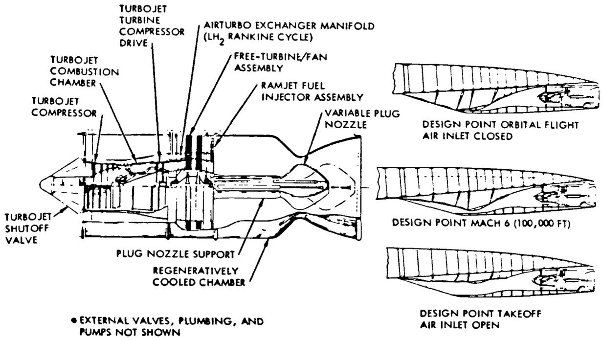
Figure 1.3-4. Multi-Cycle Airbreathing Engine and Inlet, Turbofan/Air-Turboexchanger/Ramjet
