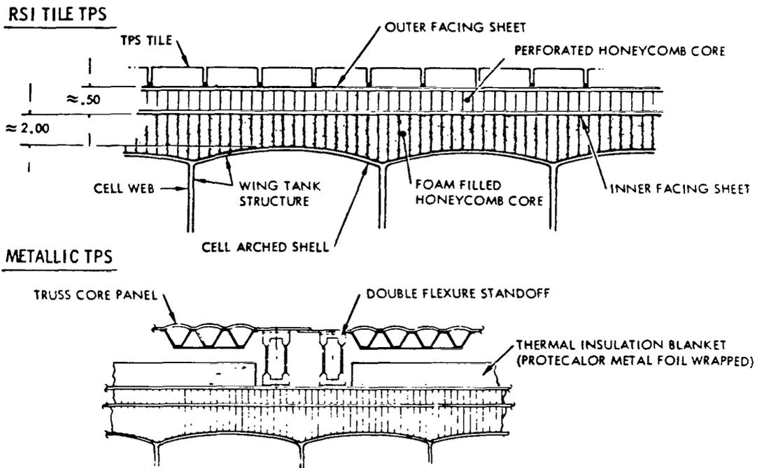
Figure 1.3-3. Wing Construction Detail with Candidate TPS Configurations
