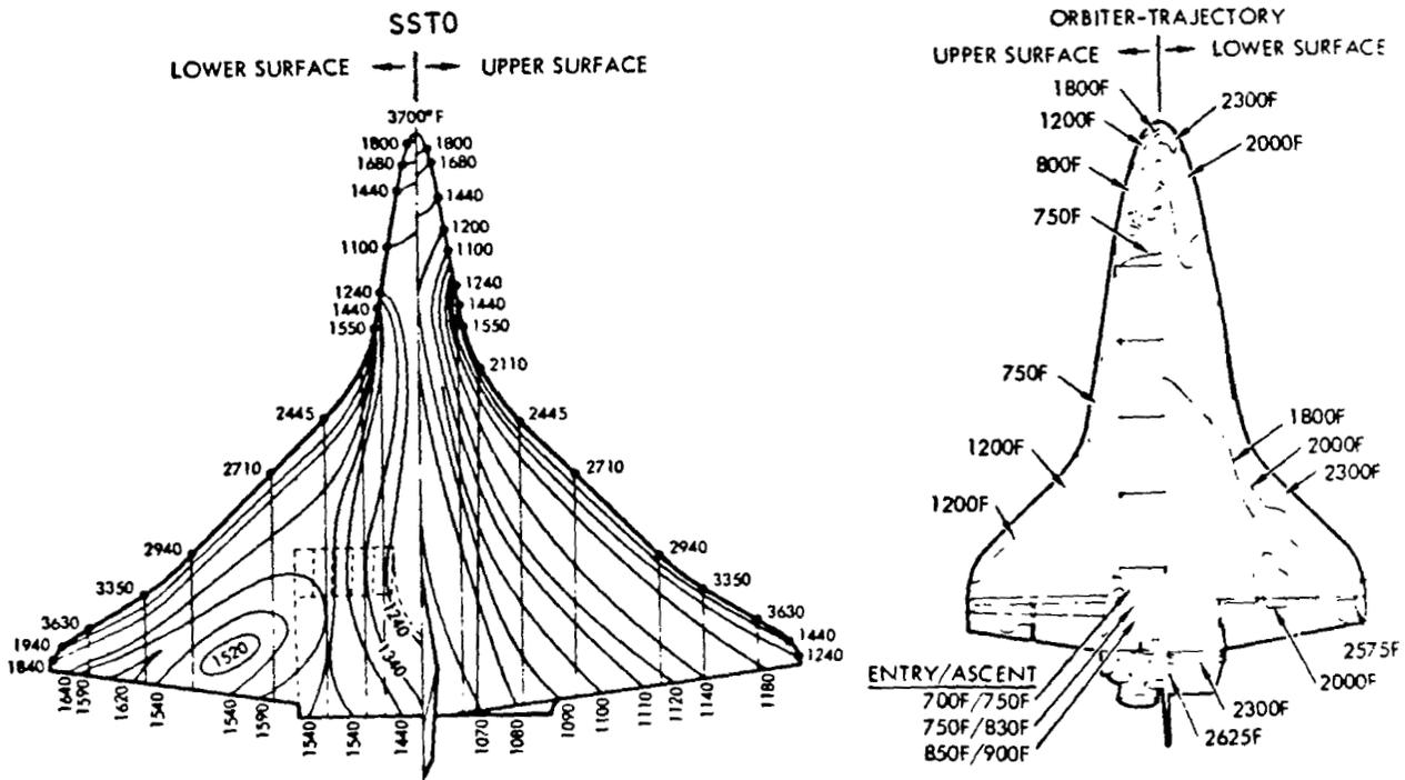
Figure 1.3-10. Isotherms of Peak Surface Temperature During Ascent
