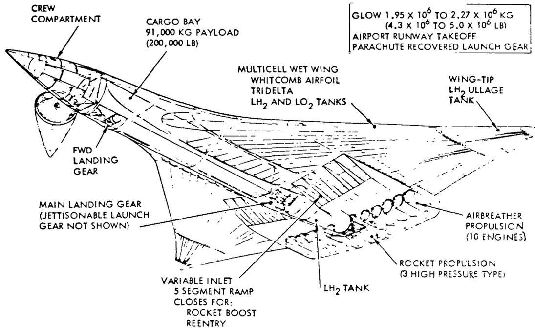
Figure 1.3-1. HTO-SSTO Design Features
