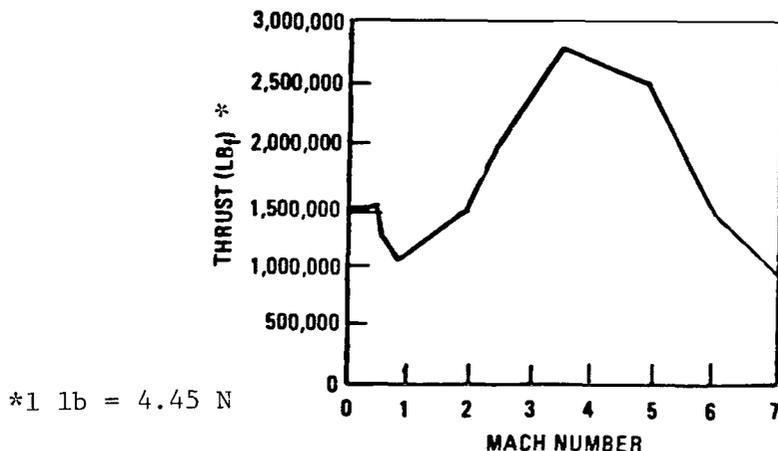
Figure 1.3-5. Airbreather Thrust Vs. Mach Number
