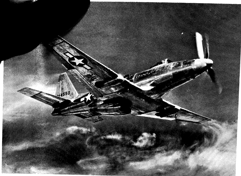
The P-75 (shown here and above is a P-75A), with its contra-rotating propeller, was a big airplane—too big, in General Bradley's opinion.
